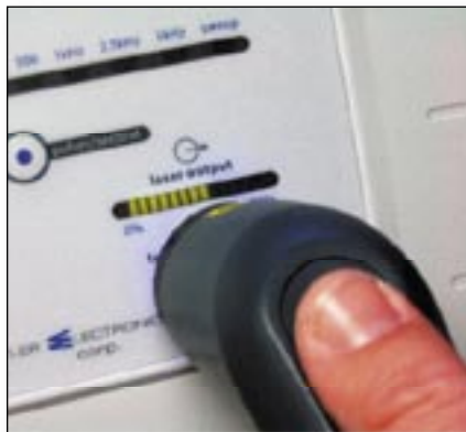
Laser applicator over laser output sensor showing visible proof of laser activity.
