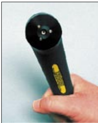
Laser Applicator showing one laser diode at 785 nm surrounded by 3 LEDs at 470 nm.
