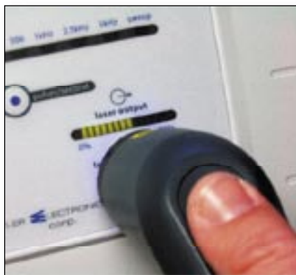
Laser applicator over laser output sensor showing visible proof of laser activity.
